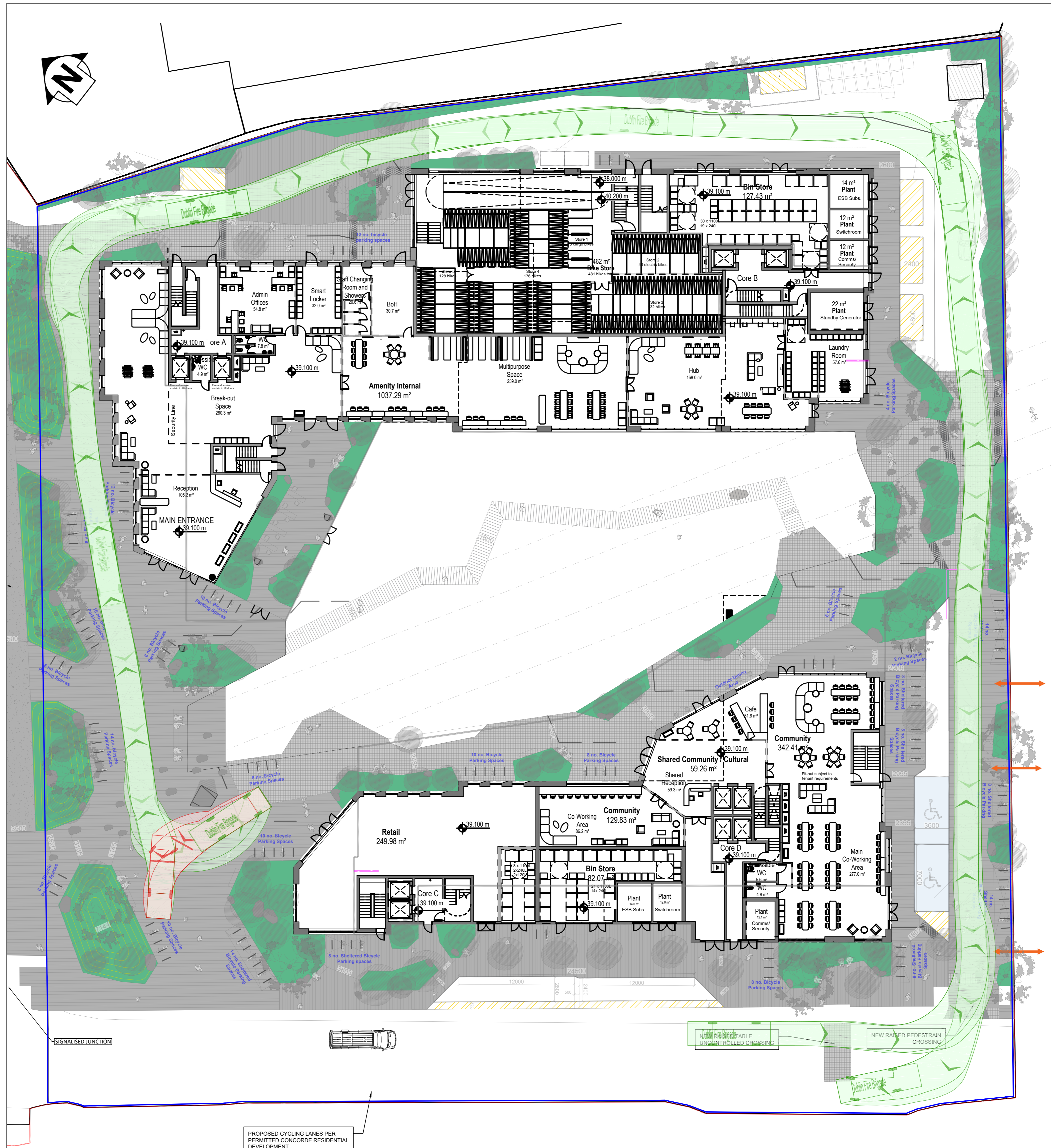
AUTOROUTE TRACKING - FIRE TENDER
